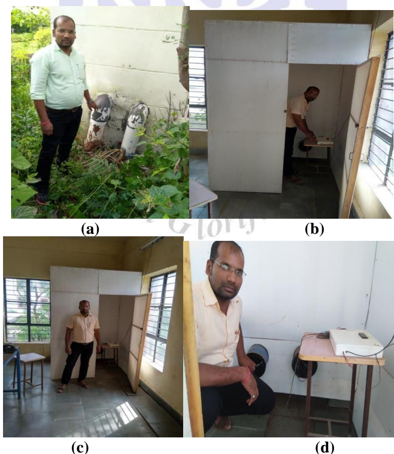
Fig1. Experimental Set Up of Earth Tube Heat Exchanger (ETHX) Installed at RKDF University (a),(b) (c) (d)
